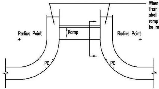
When the shared surface road is taken from a road with footways, the footways shall be extented past the top of the ramp 1.8m. A pram crossing (PC) will also be required on the radius as shown.
