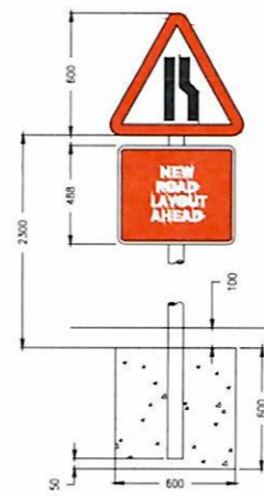
TSRGO REF 517 (ROAD NARROWS ON RIGHT AHEAD) RETROFLECTIVE SIGN (UN-ILLUMINATED) MOUNTING HEIGHT 2300mm TSRGO REF 7014 (NEW ROAD LAYOUT AHEAD - TEMPORARY) CLASS 1 RETROFLECTIVE SIGN (UN-ILLUMINATED) MOUNTING HEIGHT 2300mm POST TO BE 76mm \phi POWDER COATED TUBULAR STEEL (GREY) FOUNDATION TO BE CONCRETE MIX ST2 TS01
