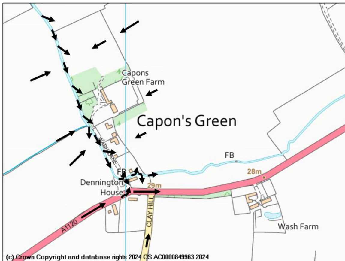
Figure 13 Approximate flood water flow paths at Capon's Green
