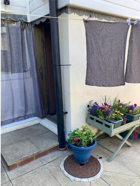
Depth of flooding externally adjacent semi-detached properties, marked by cable tie on downpipe
