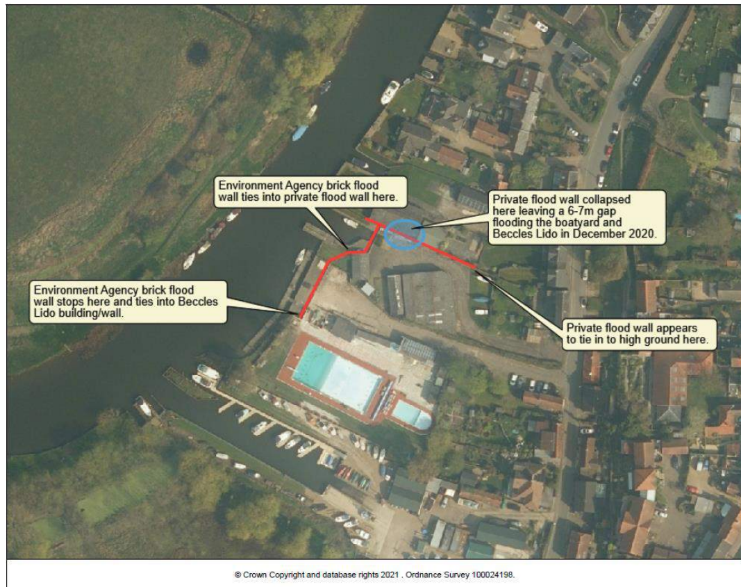
Figure 4 – Location and extent of flood wall breach (Environment Agency)
