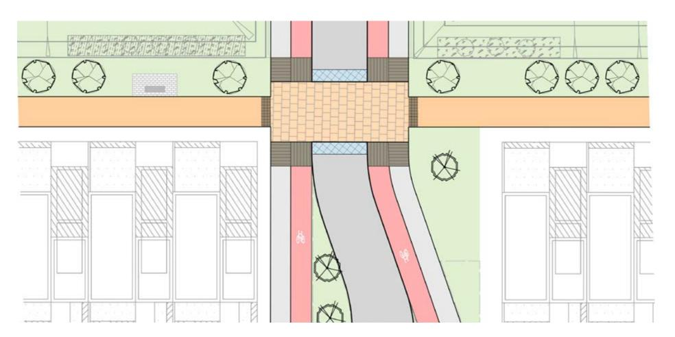
Figure 29 - Primary Pedestrian and Cycling Route Crossing Secondary Vehicular Route
