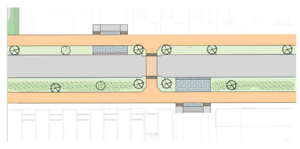
Figure 28 - Secondary Pedestrian Route Crossing Secondary Vehicular Route
