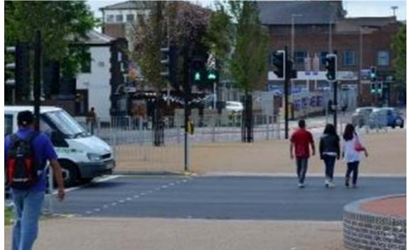
**Formalised crossings** either use road markings or signals to allow pedestrians to cross. For instance, zebra and tiger crossings are a formalised crossing that minimises the delay for pedestrians and cyclists.
