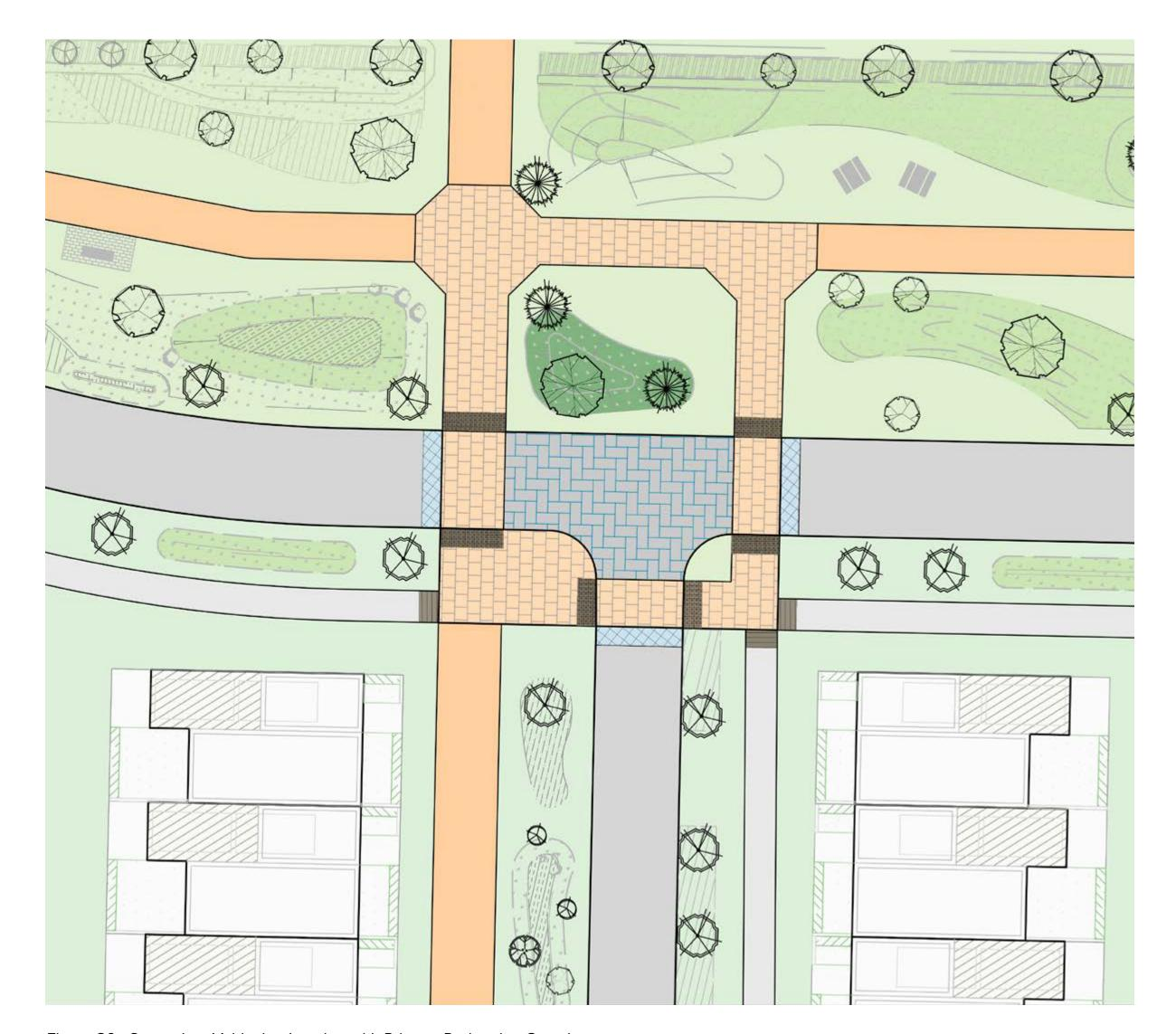
Figure 30 - Secondary Vehicular Junction with Primary Pedestrian Crossing
