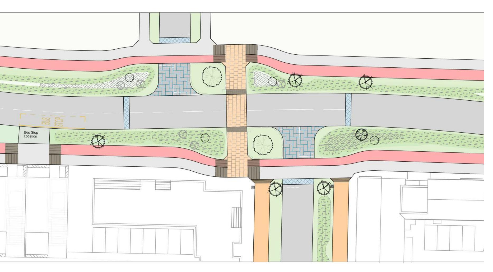
Figure 27 - Primary Pedestrian and Cyclist Crossing with Secondary Vehicular Junction
