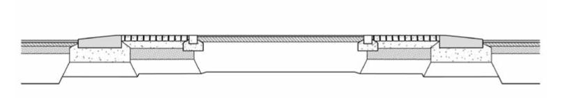
Figure 5 - Typical Cross Section of Access using Dutch Entrance Kerb
