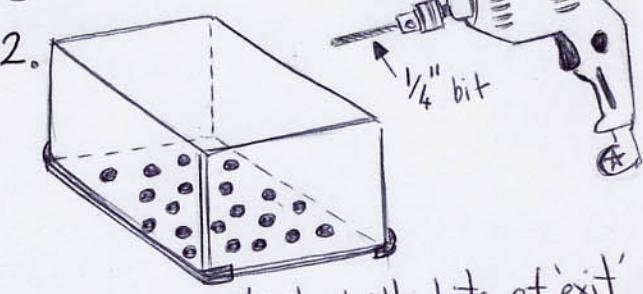
2. ...Next, drill lots of 'exit' holes in the bottom of 2 of the boxes, using a 1/4" drill bit...
