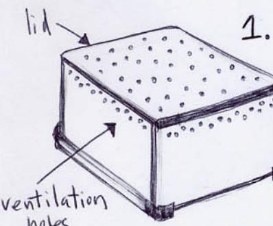
1. drill lots of tiny holes around the top of the boxes to allow for ventilation, doing the same all over the lid...
