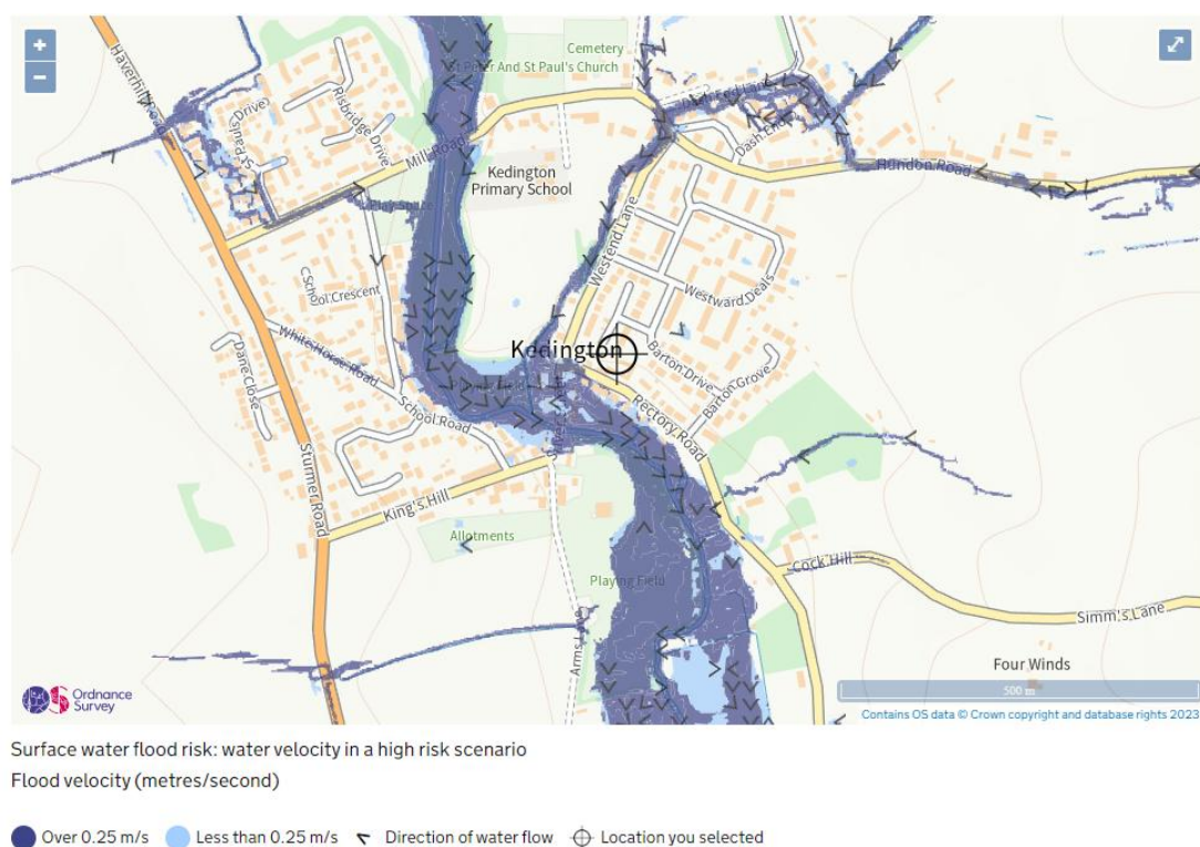
Figure 3 – Pluvial flood risk map with water velocity.
