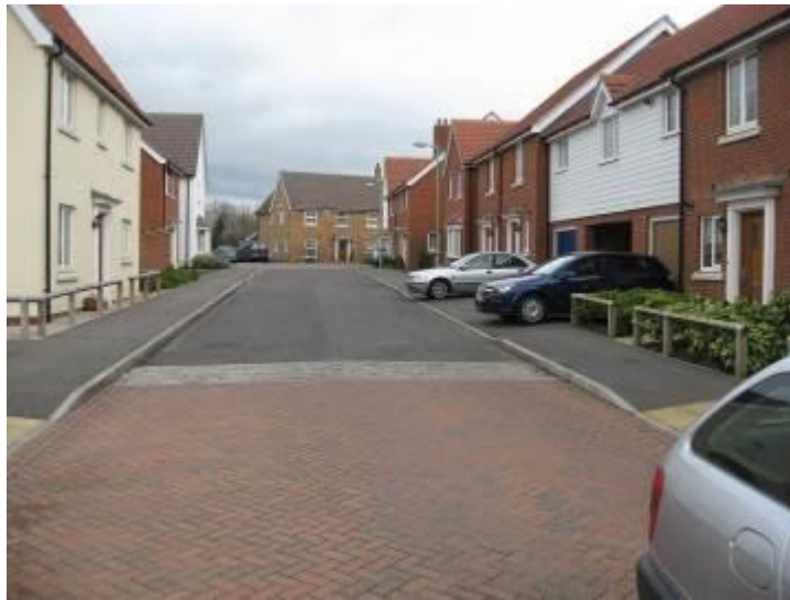
Cedars Park (Phase 4A), Stowmarket: an example to highlight the poor design with regards to cars protruding on the footway.
