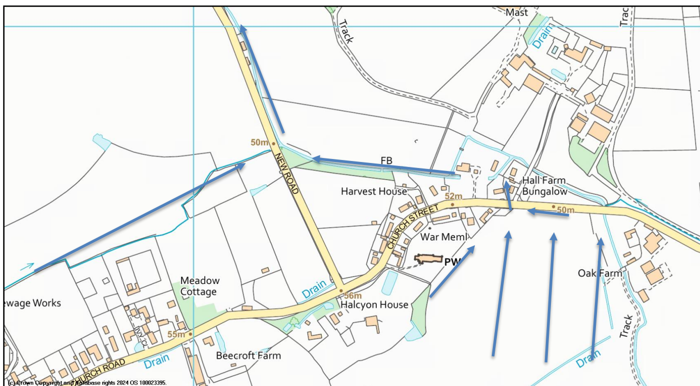
Figure 16 - Flow routes of water in east Worlingworth
