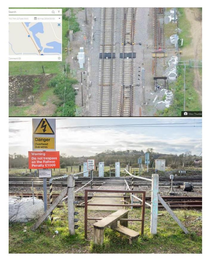
Trains on this line travel at up to 44.7m/s. The current traverse distance is 9m, which at a walking pace of 1.2m/s requires 7.6 seconds to cross. For users of the level crossing to have sufficient time to cross, it is necessary for them to be able to see a train when it is at least 338m away. Available sighting from the current decision points exceeds this in all
