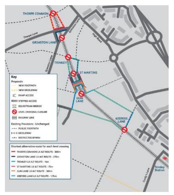
The proposed diversion at Gun Lane comprises a crossing over the bridleway bridge, which is proposed to be sited at Gun Lane.
