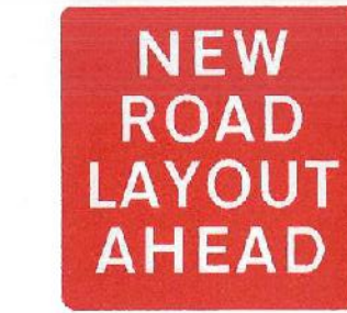
ROAD SIGN - DIAG. 7014 DIAG 7014 NEW ROAD LAYOUT AHEAD SIGN TO BE TEMPORARILY MOUNTED TO POST MIN. 45m TO MAX. 110m AHEAD OF PROPOSED WORKS LOCATION TO BE AGREED WITH S.C.C. SIGN TO BE REMOVED AFTER A PERIOD OF THREE MONTHS. REMOVAL DATE TO BE PRINTED ON REVERSE
